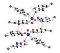
The characterization of the gadolinium complex with 5,7-dichloro-8-quinolinolato (H5,7ClQ) ligands, [Gd(5,7ClQ)<sub>2</sub>-(H5,7ClQ)<sub>2</sub>Cl], allows satisfactory interpretation of the properties of this new neutral tetrakis-type compound and points out that extensive  $\pi$ -stacking interactions affect its spectroscopic and magnetic behaviour.
